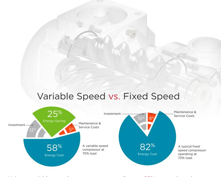
Using a variable speed compressor can easily save 25% energy by using just the right amount of energy required to do the job and no more.
