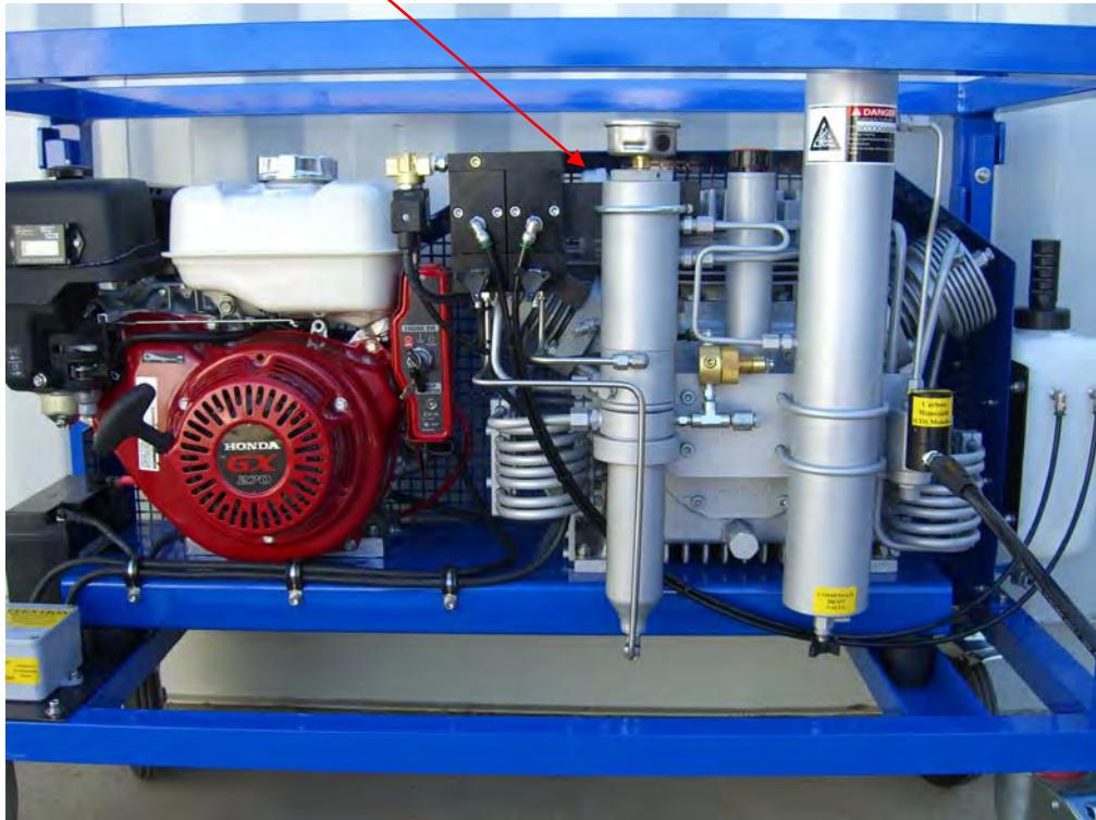
Open all manual drains while performing service! Do not hand twist gage to remove cap!
