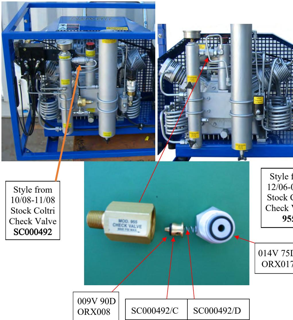
The check valve on the left is not the same as the 955 valve on right!
