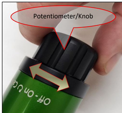
The Problem: Knob does not turn on, turn off, or calibrate the O 2 Quickstick.
