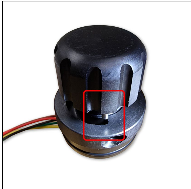
Step 4(b). Align the metal stop pin with the end of the limit stop groove. Press the knob firmly into place. Press straight down. Do not twist. Rotate knob clockwise. A click, indicating the switch turning on, should be heard.
