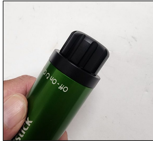
Step 3(a): Replace knob. Increased split shaft tension should make knob work. If not, try Steps 1–3 again. Still not working? Contact ron@nuvair.com for assistance.
