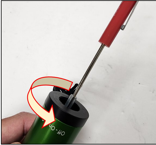
Step 2: Use small screwdriver to gently spread knob split shaft. Turn screwdriver counterclockwise only.
