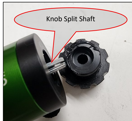
Step 1: Remove knob to expose knob split shaft. Pull straight out. Do not twist.
