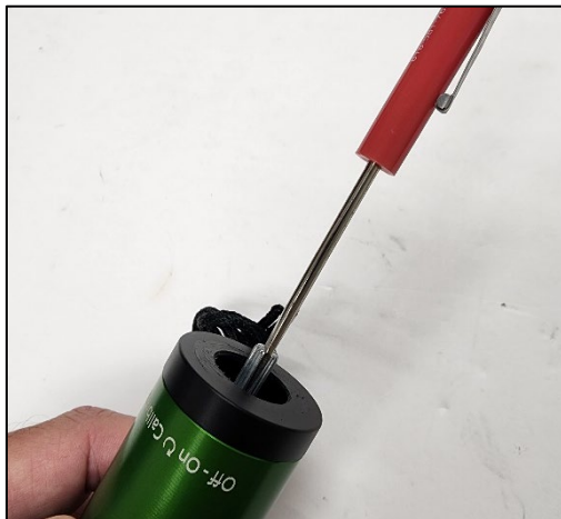
Use small screwdriver to gently spread knob split shaft.
