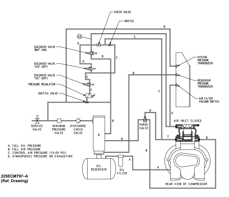
FIGURE 4–9 – CONTROL SCHEMATIC – COMPRESSOR UNLOADED – CONSTANT SPEED MODE EBH & EBM UNITS ONLY
