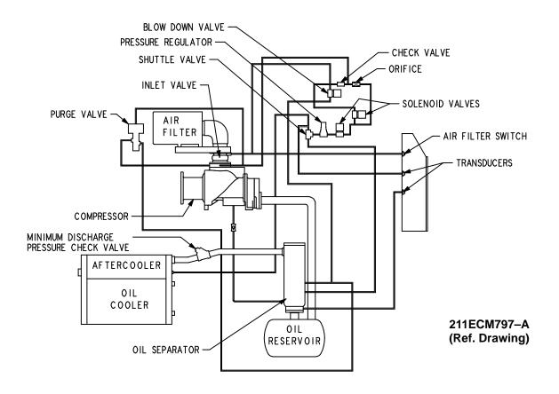
FIGURE 4–3 – SCHEMATIC TUBING DIAGRAM
