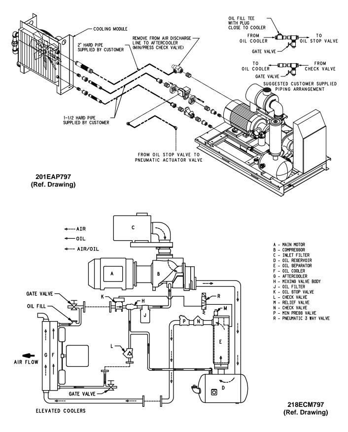
FIGURE 5–2 – OIL FLOW DIAGRAM – REMOTE OVERHEAD MOUNTED
