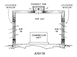
FIGURE 2–1 – TYPICAL COMPRESSOR ROOM
