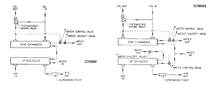
\* (OPTIONAL) WATER CONTROL VALVE AND WATER SHUTOFF VALVE MUST BE ORDERED SEPARATELY.
