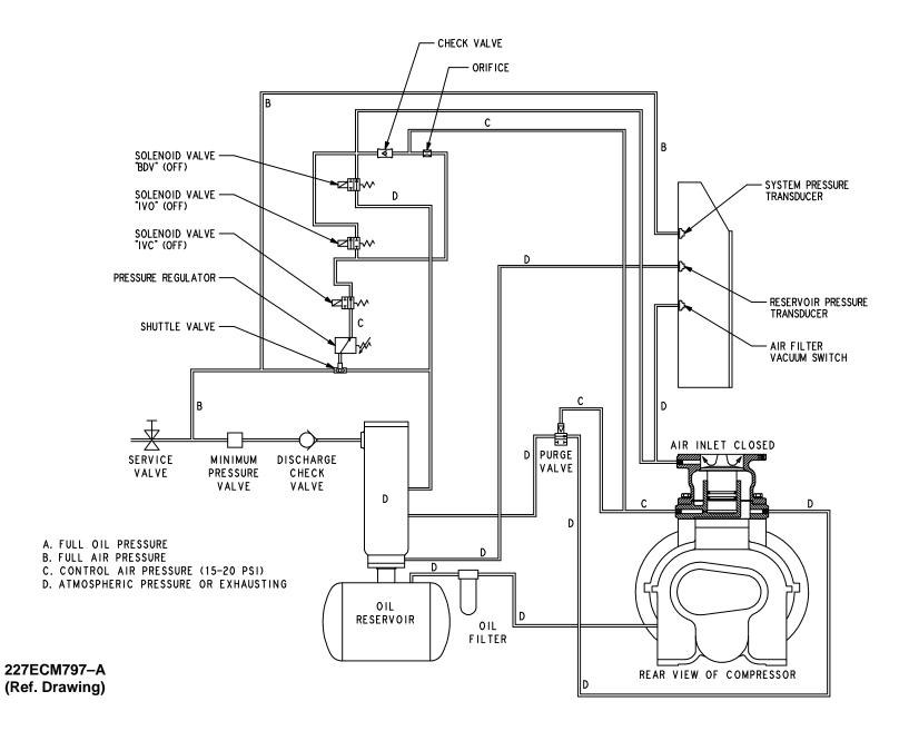
FIGURE 4–11 – CONTROL SCHEMATIC – COMPRESSOR UNLOADED – LOW DEMAND MODE OR AUTO MODE EBH & EBM UNITS ONLY
