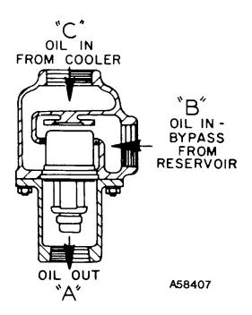
FIGURE 5-7 - THERMOSTATIC MIXING VALVE ELEMENT
