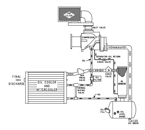
FIGURE 1-6 - PACKAGE - AIR/OIL FLOW DIAGRAM
