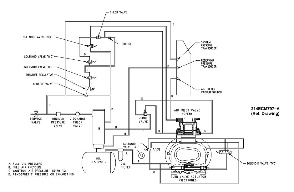
FIGURE 4–12 – CONTROL SCHEMATIC – COMPRESSOR AT FULL LOAD EAP UNITS ONLY
