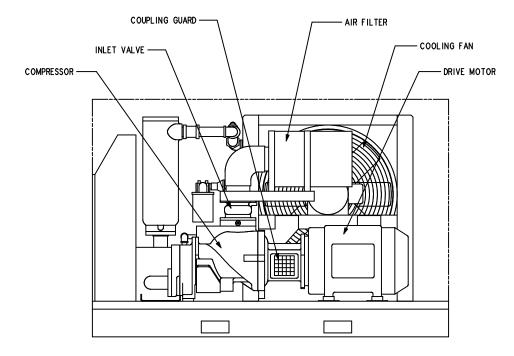
FIGURE 1–4 – PACKAGE – DRIVE MOTOR & AIR FILTER
