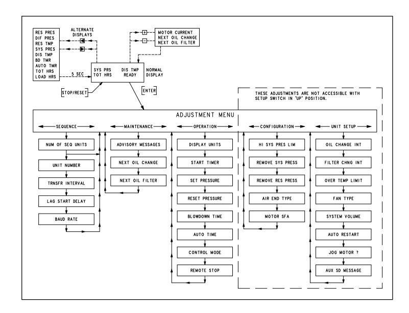
FIGURE 4–2 – FLOW CHART FOR SET–UP PROGRAMMING AUTO SENTRY–ES+
