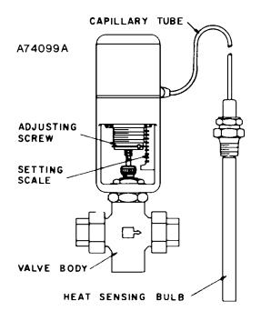
FIGURE 5-8 - WATER CONTROL VALVE
