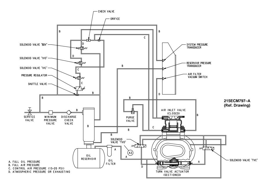
FIGURE 4–13 – CONTROL SCHEMATIC – COMPRESSOR FULLY UNLOADED – LOW DEMAND MODE SWITCH OFF EAP UNITS ONLY
