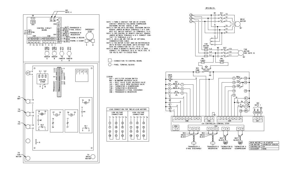
FIGURE 4–15 – WIRING DIAGRAM – 214ECP546 (WYE–DELTA – EBM & EBP UNITS ONLY)
