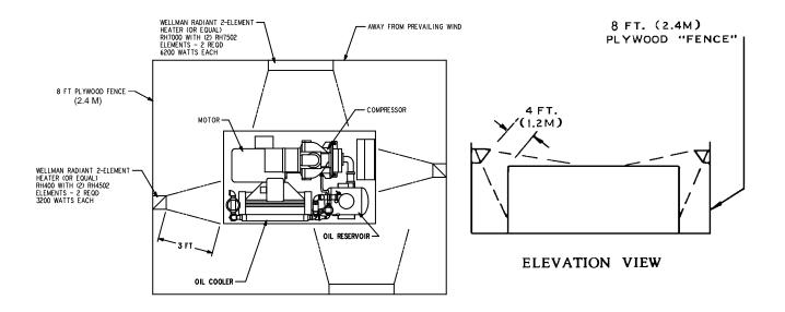
FIGURE 2-3 - COLD WEATHER INSTALLATION
