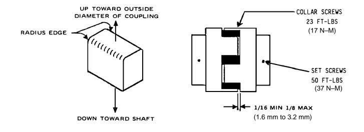
FIGURE 7-1 - INSTALLATION OF COUPLING CUSHIONS
