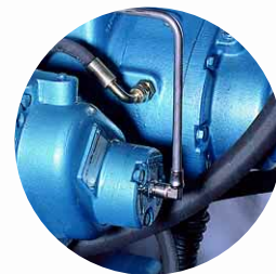
Thrust balance pistons on low and high pressure compression elements equalise bearing loads and extend element life
