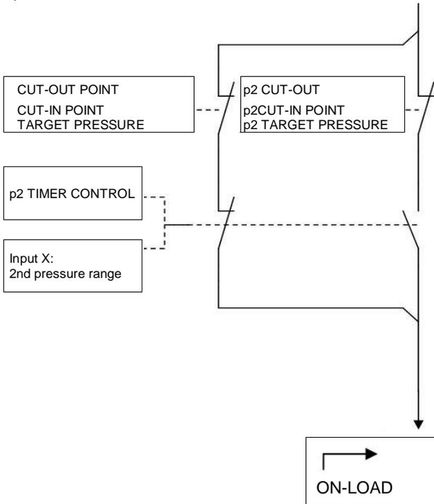
Fig. 3 Remote Pressure Changeover.
