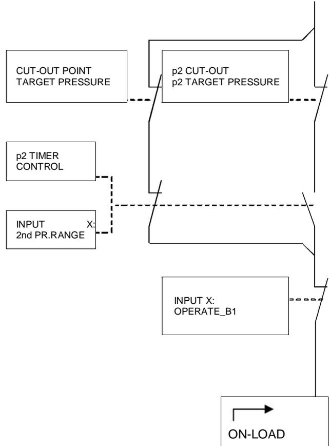
Fig. 4 On-load/Off-load Remote Control
