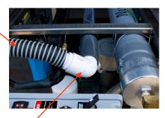
Attach this end of hose to Nitrox System outlet Attach the other end of hose to compressor intake
