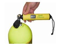
Use independent oxygen analyzer for verification
