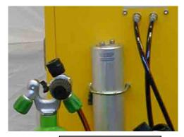
Fill Whip Attached to Scuba Cylinder
