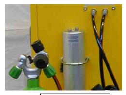
Fill Whip Attached to Scuba Cylinder
