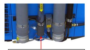
Attach one end of the suction hose here and the other end to the compressor intake.
