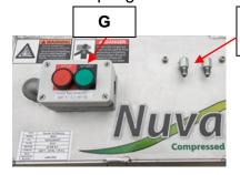
Fill Whip connection points on compressor
