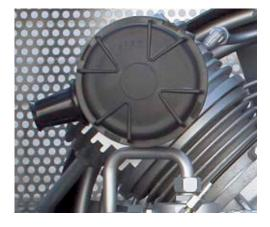
The air intake filter must be changed every 250 working hours or annually. If the compressor is used in a dusty environment the filter change interval should be reduced to every 100 hours. Change the Air filter as follows:
