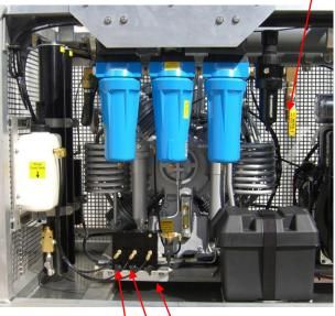
Manual Condensate Drain Valves (3X)
