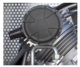
The air intake filter must be changed every 250 working hours or annually. If the compressor is used in a dusty environment the filter change interval should be reduced to every 100 hours. Change the Air filter as follows:
