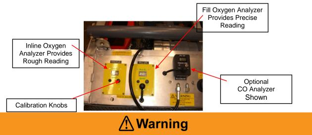
Oxygen analyzers must be calibrated before each use. See oxygen analyzer manuals for correct calibration procedures. Improper calibration of the fill oxygen analyzer may result in the use of incorrect nitrox mixtures, which may cause serious injury or death to the diver using the gas mixture.
