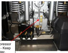
Check HP Compressor Lubricant Level - Keep Level in Center.
