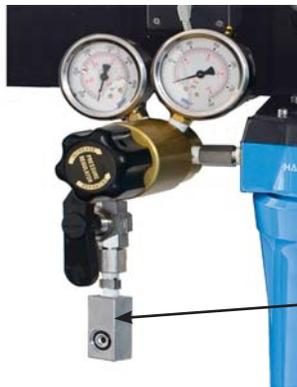
Attach HP Supply Air to On/Off Flow Valve Fitting
