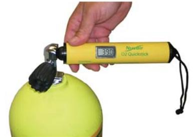
Use Independent Oxygen Analyzer for Verification
