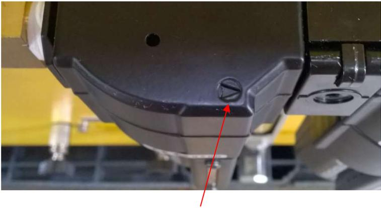
Air Flow Direction: The direction of air flow is shown by a stamped arrow.
