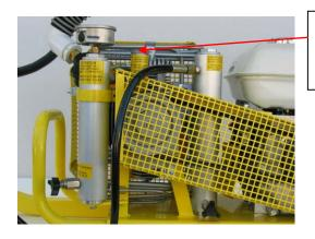
Oil Cap with Dipstick -Keep Lubricant Level between Min and Max Marks on Dipstick.
