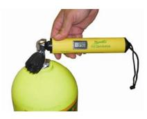
Use Independent Oxygen Analyzer for Verification
