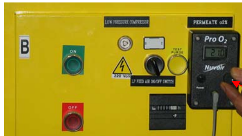
Permeate Oxygen Analyzer Provides Rough Reading
