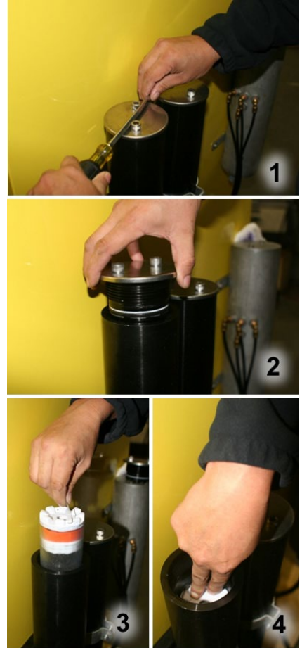
Figure 24. Changing air filter cartridge.
