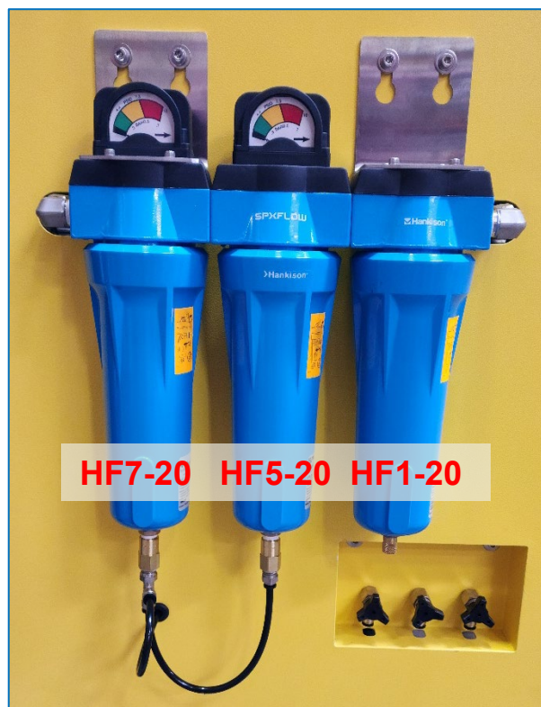
Figure 21. Low pressure filtration and drain valves.
