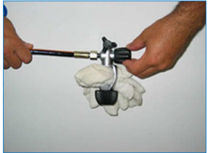
Figure 15. Clean rag acts as sound muffler.
