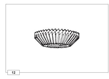
After prolonged running of the engine the hammering of the valves on their seats at high temperature tends to harden the faces of the seats and makes manual grinding difficult. It is necessary to remove the hardened surface with a 45° cutter (fig. 12).
