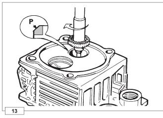
Grinding of valve seats causes a widening of the valve seat face **P** (fig.13).
