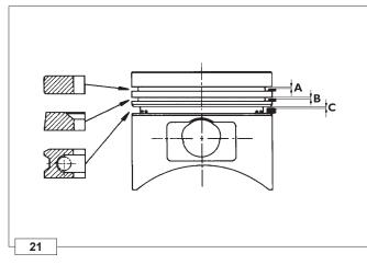
Check that the rings move freely in the grooves and check the ring/groove clearance using a feeler gauge (fig.21).
