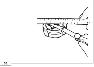
The clearance between the external rotor of the oil pump and the cover facing surface must be:
