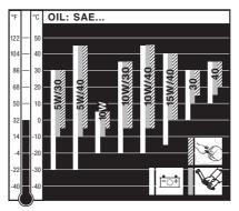
Choose the recommended viscosity based on the type of start (recoil, crank handle or electric) and on the engine temperature at which the engine will be operated.
