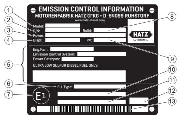
The layout of the EPA/CARB type plate depends on the engine application and is affixed to the sound protection hood. It contains the following information:
