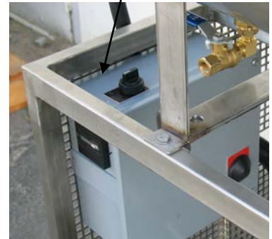
On/Off LP Feed Air Supply Valve Handle in Open Position
