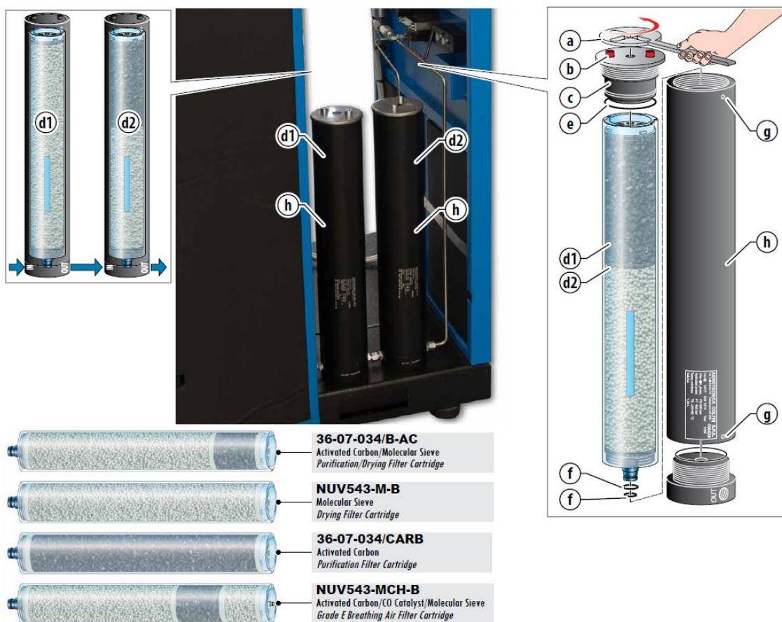
Figure 29. Air filter changing diagram.
