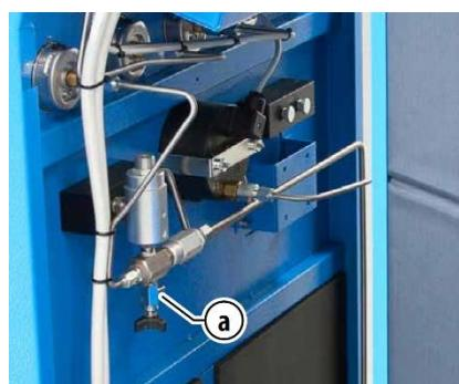
*Figure 20. Opening drain valve depressurizes system.*
