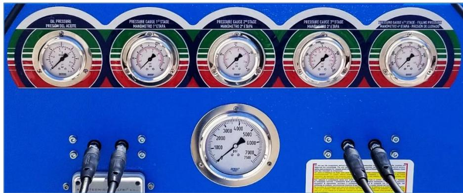
Figure 17. Oil, interstage, and final pressure gauges.
