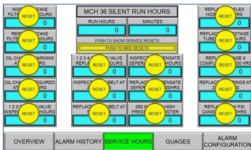
Figure 7. Service Hours screen showing reset buttons.
